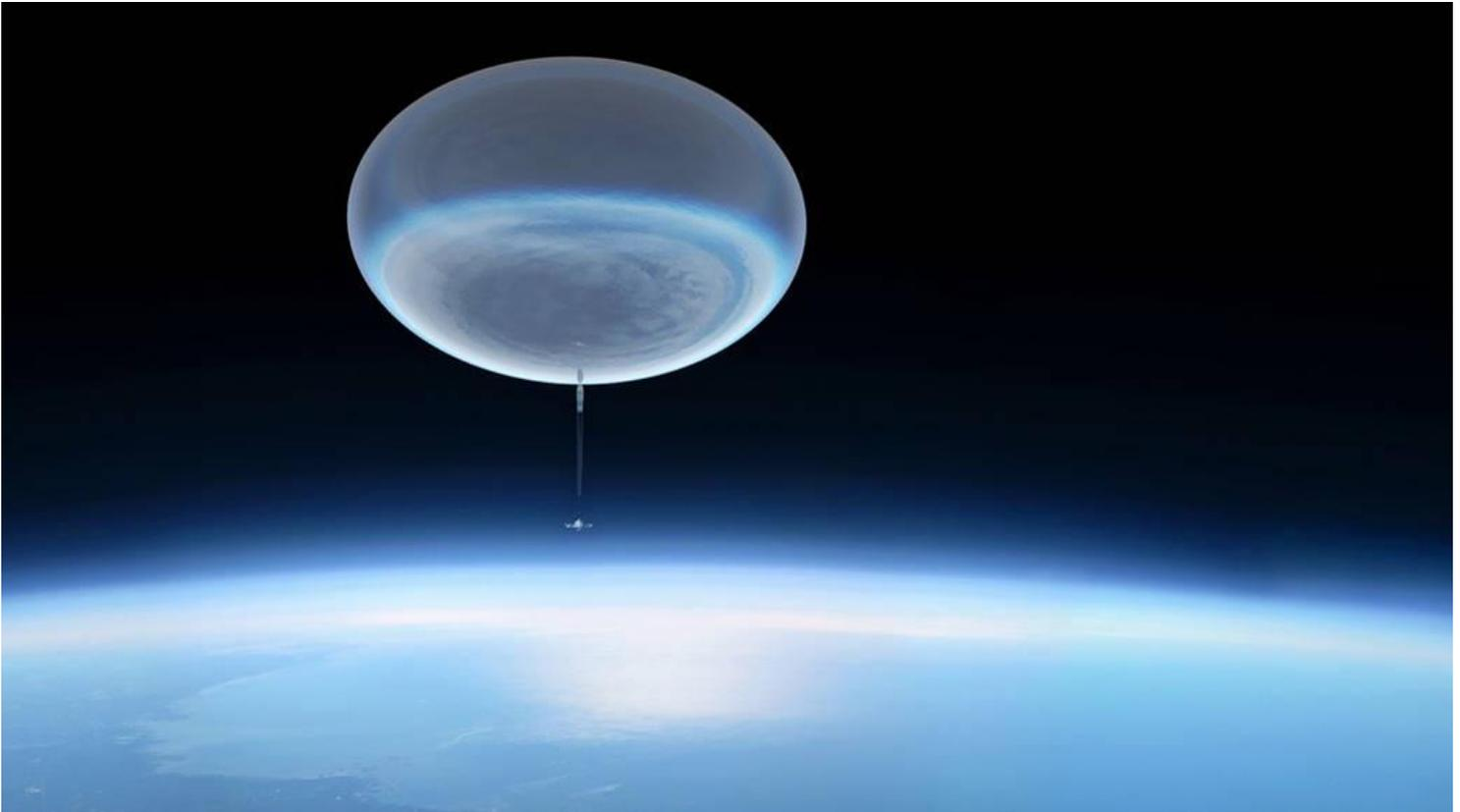
Carried high into the stratosphere by a balloon the size of a football stadium, the ASTHROS telescope will observe wavelengths of light that are not visible from the ground. The launch is planned for December 2023, from Antarctica.
