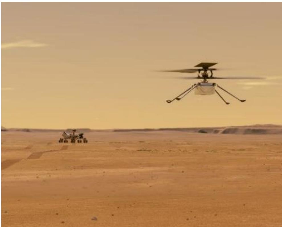
*After a successful first flight on 19 April 2021, NASA's Ingenuity Mars Helicopter showed that powered flight is possible on the Red Planet. The Ingenuity experiment will explore how aerial scouting could benefit future exploration of Mars and other celestial bodies.
